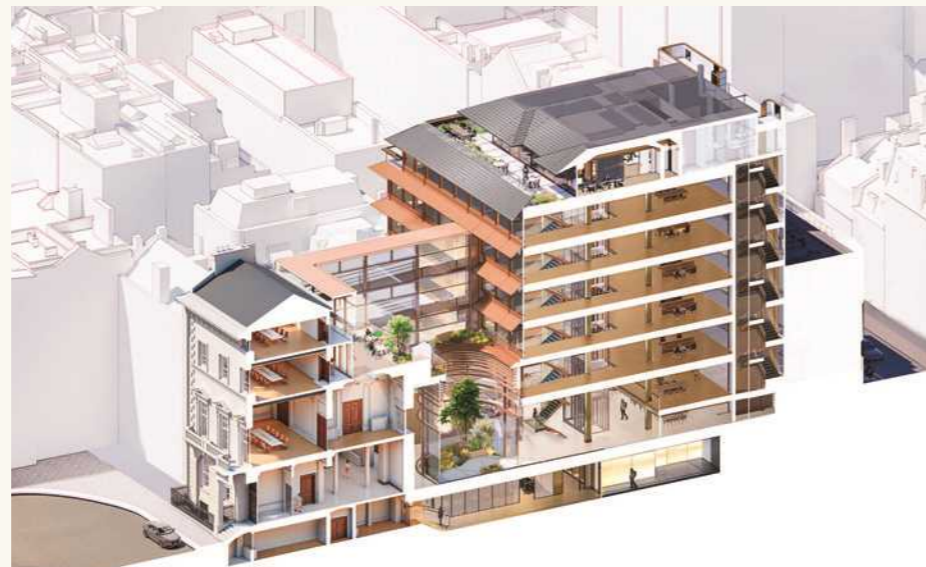
Proposed cross-sectional view showing the new multi-level walkways connecting the modern block with the historic townhouse at no 11.
